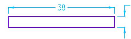
1" THICK EPOXY BACK SPLASH FRONT FACE, TOP, LEFT, & RIGHT EDGES ARE FINISHED
